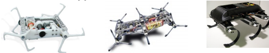
Figure 1. Robot with wheg concept: a) Mini-Whegs b) WHEGS I [7] and c) Edubot [8,9]
